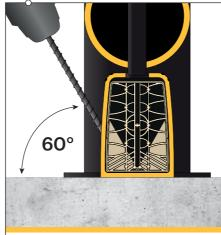
Retro fit installation 60° diagonal fixing method allows a fast and easy retro-fit to any existing barrier system
